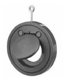
STAFFORD CHECK VALVE MODEL SERIES - 40 ARE PRIMARILY SINGLE PLATE SWING CHECK VALVE WITH A SHORT PATTERN BODY CONFORMING TO THE API 6D AND ANSI B16.10 FACE TO FACE DIMENSIONS.
